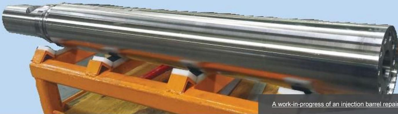
A work-in-progress of an injection barrel repair.
